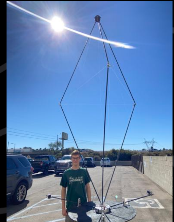
4 meter tensegrity tower deployed with intern for scale.
